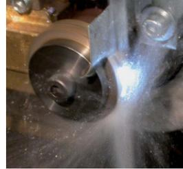
*Contact-free truing of metallic-bonded grinding wheels*
